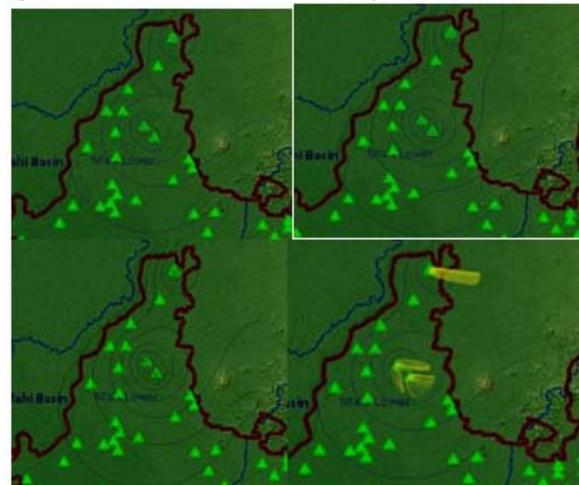
Fig. 3. Effect of well abstraction on ground water head in basalt system for NHS in Savli for (a) 30lps (b) 35lps (c) 40lps (d) maximum area contributing to well
