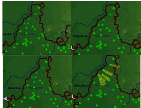
**Fig. 2. Effect of well abstraction on ground water head in older alluvium system for NHS in Savli for (a) 30lps (b) 35lps (c) 40lps (d) maximum area contributing to well**
