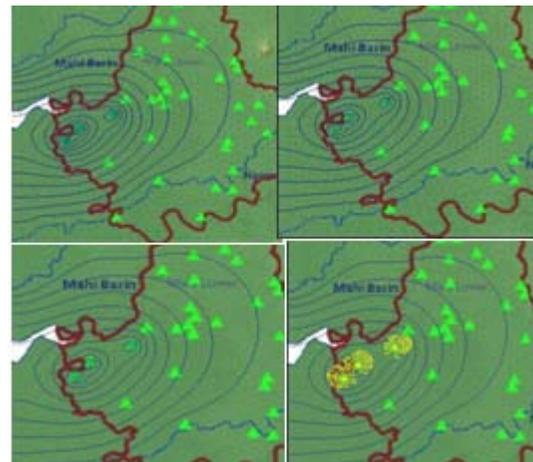
Fig. 6. Effect of well abstraction on ground water head in coastal alluvium for NHS in Padra for (a) 30lps (b) 35lps (c) 40lps (d) maximum area contributing to well
