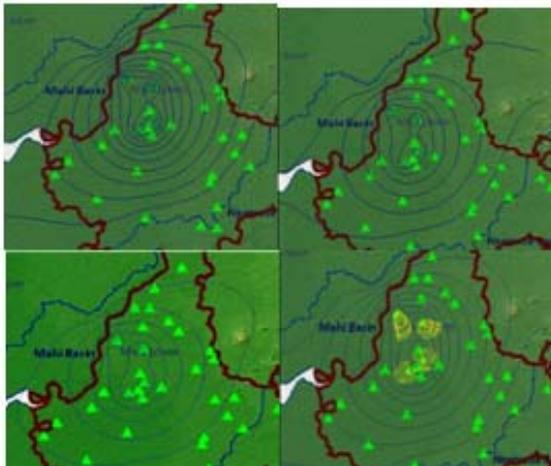
Fig. 4. Effect of well abstraction on ground water head in older alluvium system for NHS in Vadodara for (a) 30lps (b) 35lps (c) 40lps (d) maximum area contributing to well
