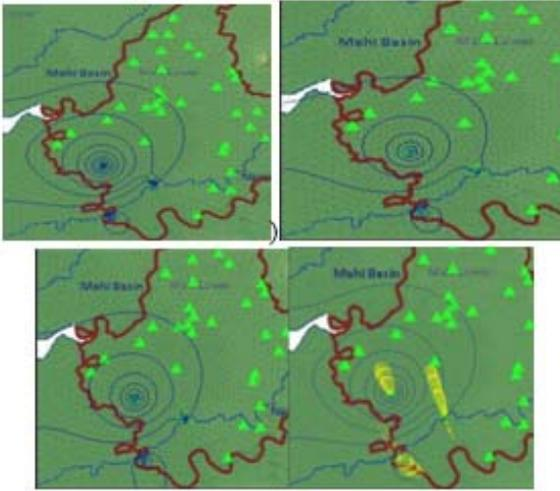
Fig. 7. Effect of well abstraction on ground water head in coastal alluvium for NHS in karjan for (a) 30lps (b) 35lps (c) 40lps (d) maximum area contributing to well
