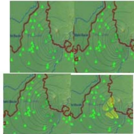
Fig. 9. Effect of well abstraction on ground water head in Basalt for NHS in Waghodia for (a) 30lps (b) 35lps (c) 40lps (d) maximum area contributing to well
