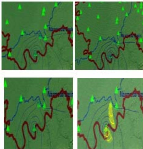
Fig. 8. Effect of well abstraction on ground water head in Younger Alluvium for NHS in Sinor for (a) 30lps (b) 35lps (c) 40lps (d) maximum area contributing to well
