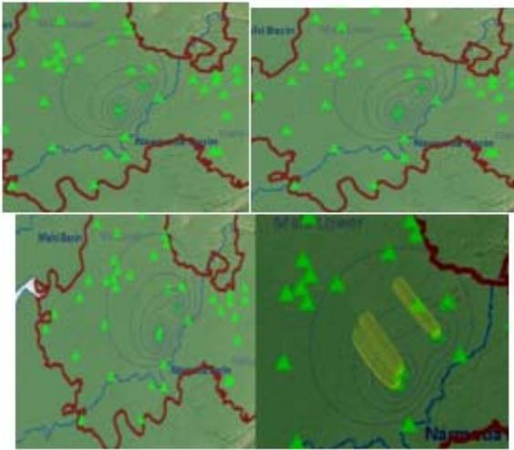
Fig. 10. Effect of well abstraction on ground water head in basalt aquifer system for NHS in Dabhoi for (a) 30lps (b) 35lps (c) 40lps (d) maximum area contributing to well
