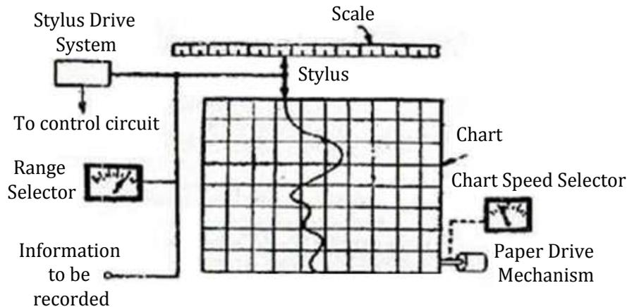
Figure 6.2 Basic strip chart recorder
