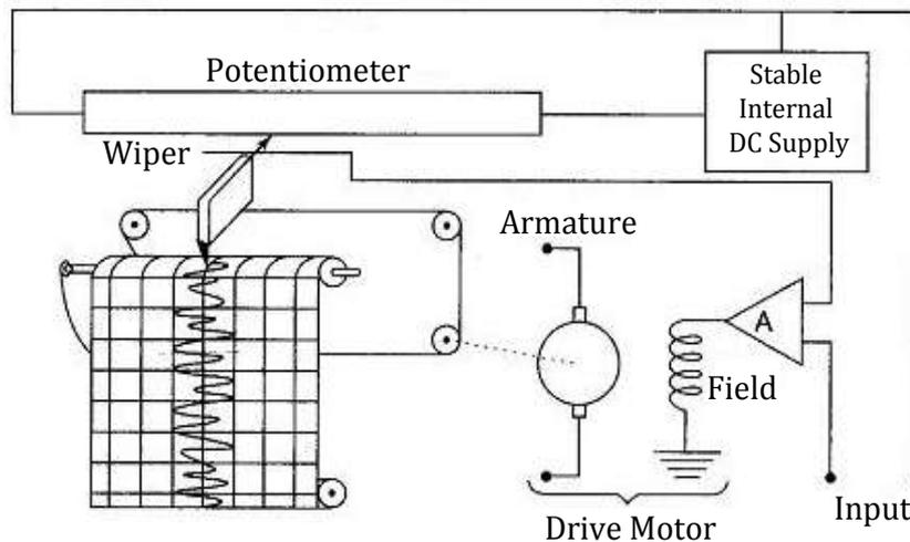
Figure 6. 4 Potentiometric type recorder
