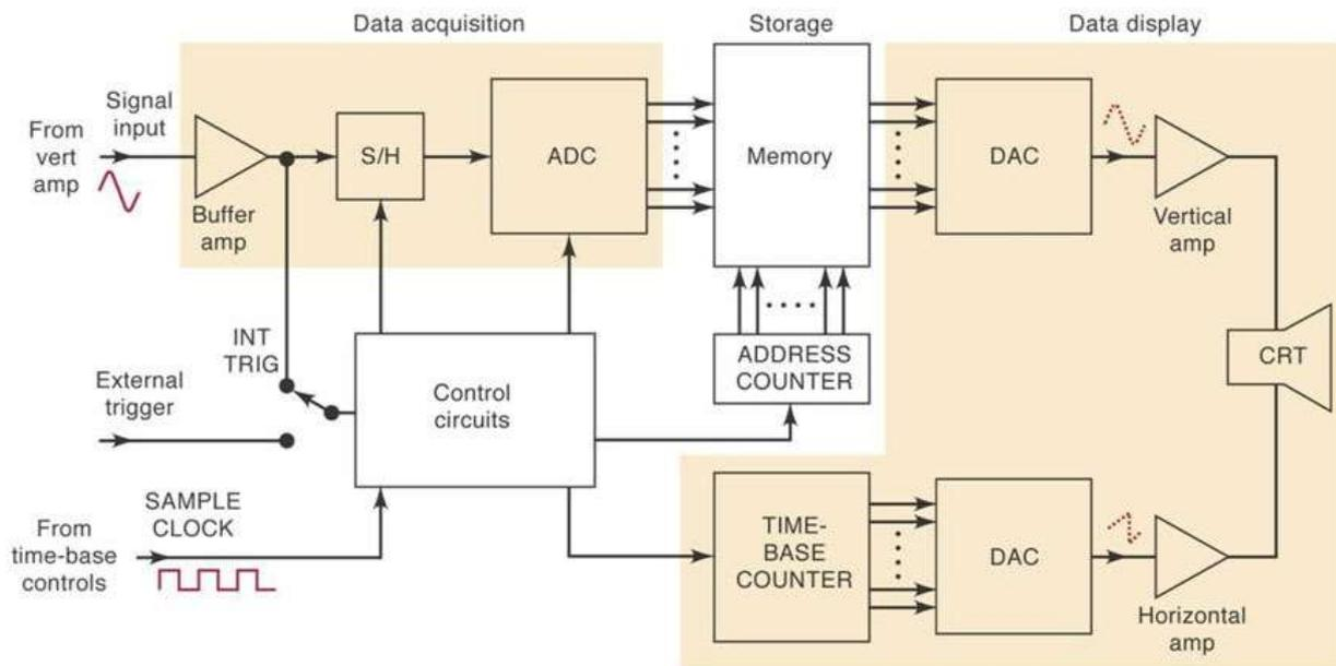
Figure 6. 7 Block diagram of Digital Storage Oscilloscope (DSO)
