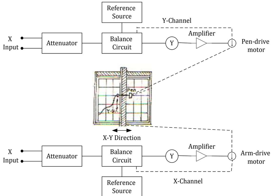
Figure 6. 5 Block diagram of a typical X-Y recorder
