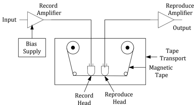
Figure 6. 6 Elementary Magnetic Tape Recorder
