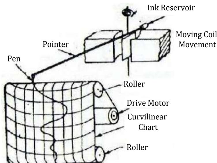
Figure 6.3 Galvanometer type strip chart recorder
